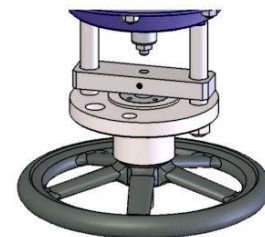
Manual Override for pneumatic actuator
